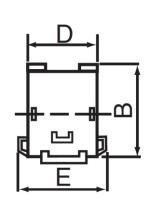
A=  $28.0 \pm 1.0 \text{ mm}$ B=  $32.0 \pm 1.0 \text{ mm}$ C=  $11.5 \pm 0.3 \text{ mm}$ D=  $18.0 \pm 1.0 \text{ mm}$ E=  $24.0 \pm 1.0 \text{ mm}$
